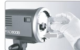
2. Match the flash tube in the Tube Socket. Push the flash tube in until it is securely seated into the socket.
